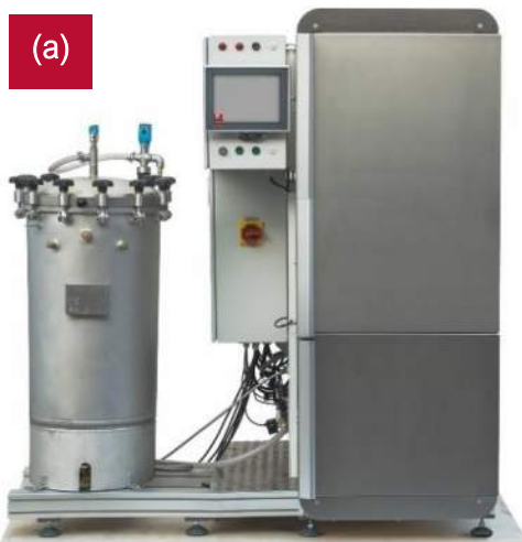
Figure 12: Delamination testing machine.
