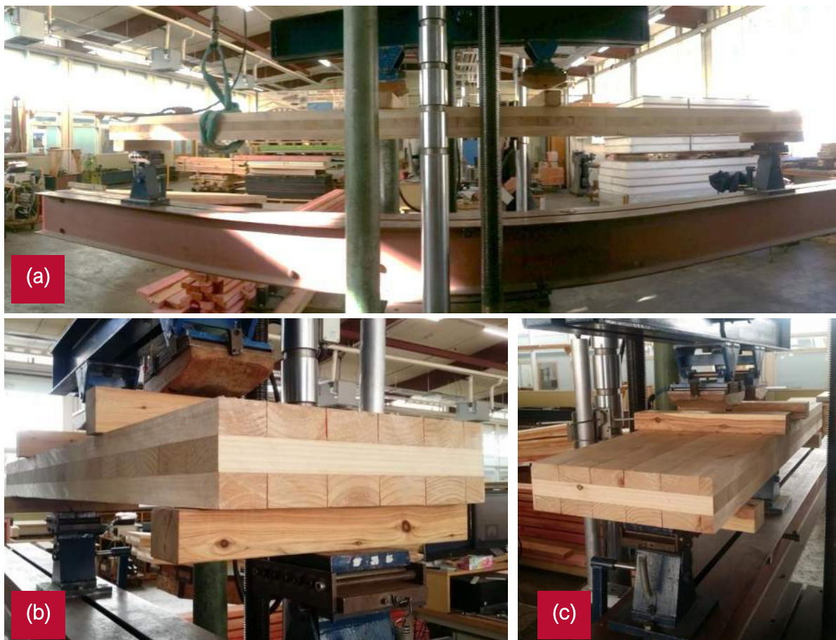
Figure 8: Large scale mechanical testing conducted by SCION; (a) Long span testing, (b) Median span testing, (c) Short span testing.
