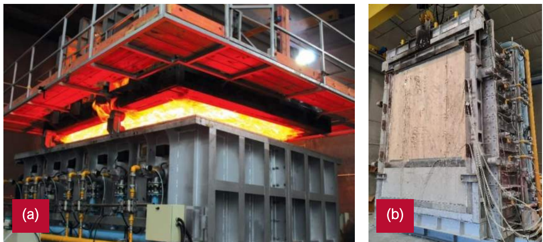
Figure 10: Large-scale fire test specimen set-up for the fire testing on Red Stag CLT; (a) Red Stag CLT floor test specimen after fire testing, (b) Red Stag CLT wall test specimen before fire testing.
