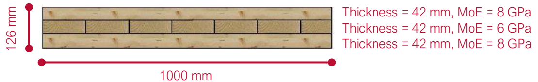
Figure 73: Red Stag CLT Panel Cross-Section
