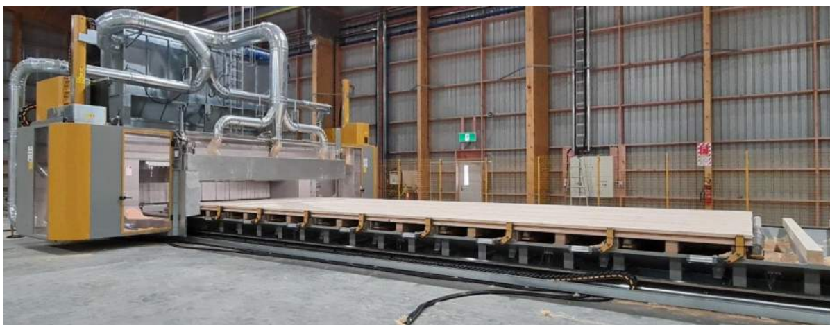
Figure 70. CNC equipment with precise cutting capability.
