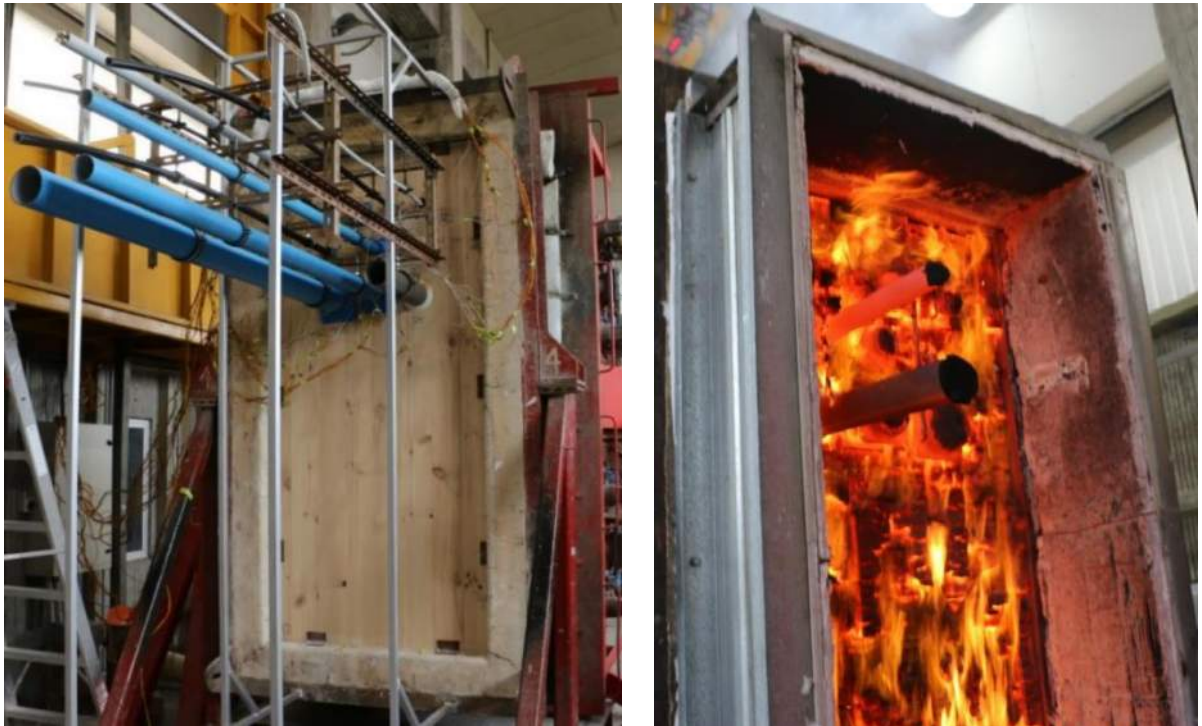
Figure 66. Various service (pipes and cables) fire tests on Red Stag CLT wall panels [26]. a) Specimen before the fire test, b) Specimen after the fire test.
