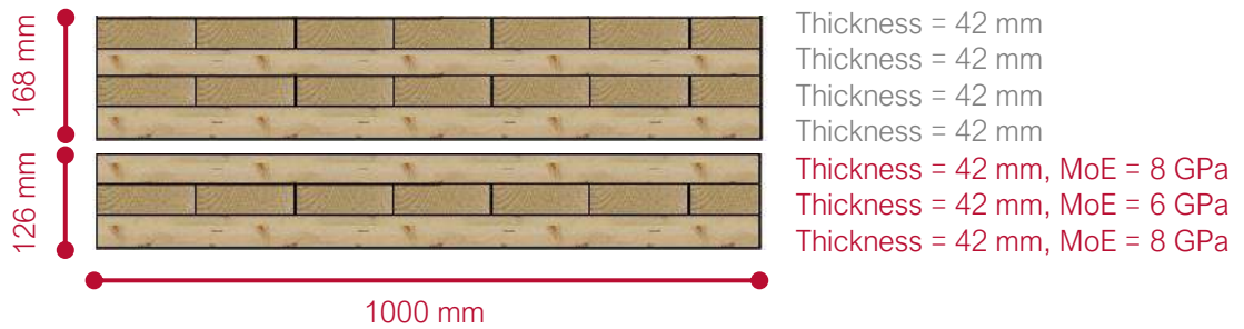
Figure 85: Red Stag CLT Panel Cross-Section
