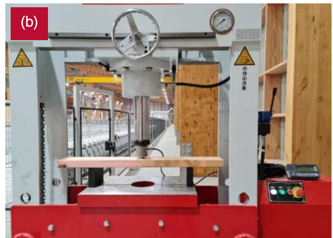
Figure 13: Finger joint test equipment and setup.
