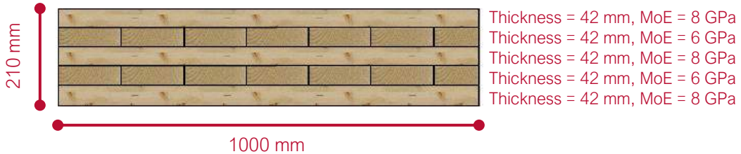
Figure 79: Red Stag CLT Panel Cross-Section
