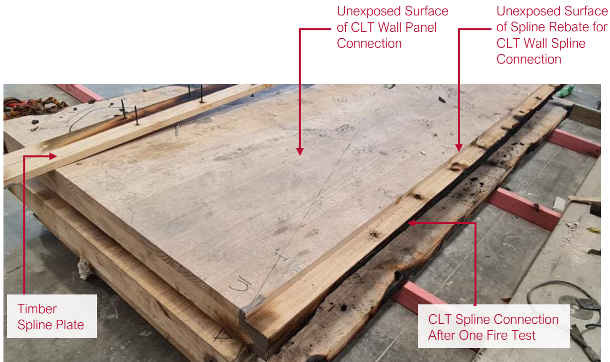
(b) Figure 62. Large-scale Red Stag CLT wall fire test set-up after testing under structural loading to test CLT connections.
