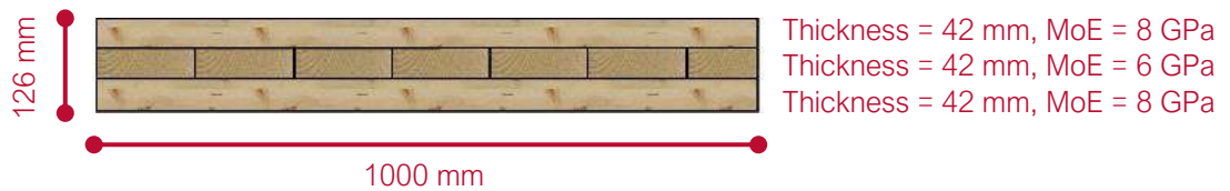
Figure 83: Red Stag CLT Panel Cross-Section
