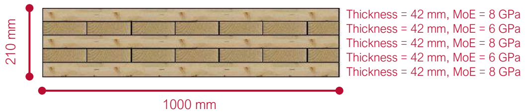
Figure 77: Red Stag CLT Panel Cross-Section
