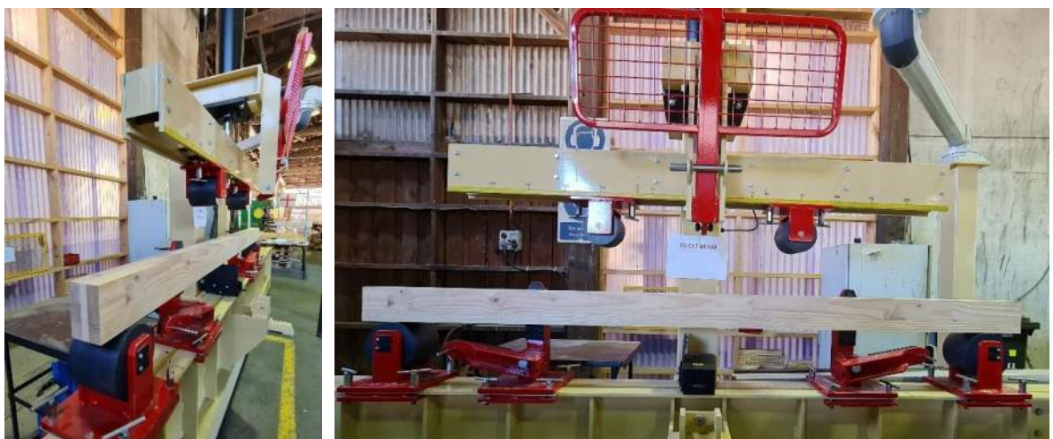
Figure 14: CLT beam bending testing machine and setup; (a) Isometric end elevation; (b) Front elevation.
