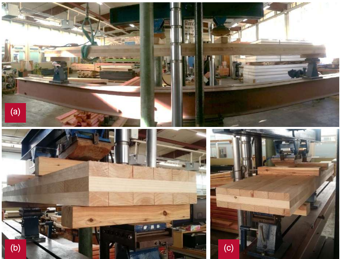
Figure 79: Large scale mechanical testing conducted by SCION; (a) Long span testing; (b) Medium span testing; (c) Short span testing.
