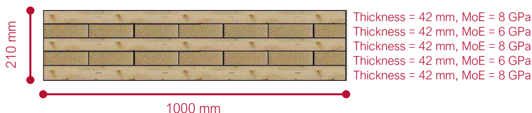
Figure 103: Red Stag CLT Panel Cross-Section
