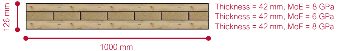
Figure 107: Red Stag CLT Panel Cross-Section
