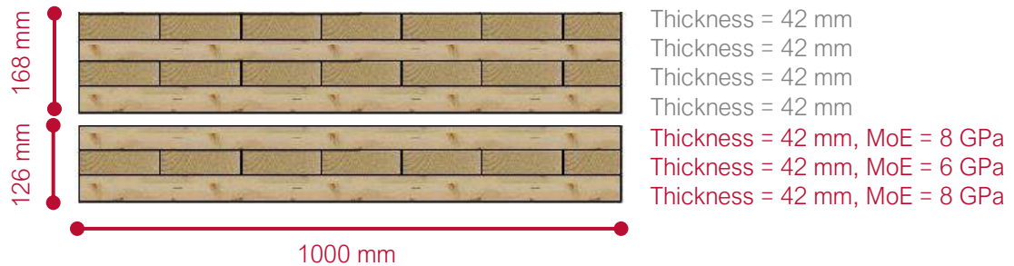
Figure 105: Red Stag CLT Panel Cross-Section
