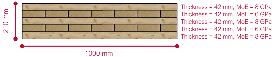
Figure 101: Red Stag CLT Panel Cross-Section
