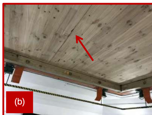
Figure 114: 210 mm thick five-layer Red Stag CLT panel with lap joint installed in the acoustic chamber at the testing laboratory.
