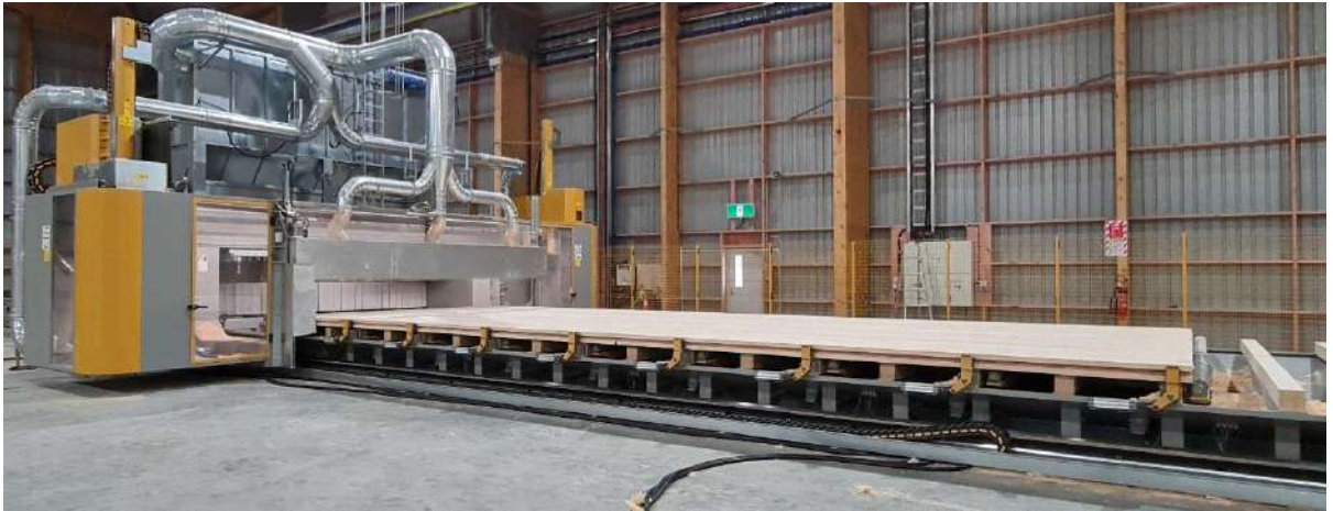
Figure 70: CNC equipment with precise cutting capability.
