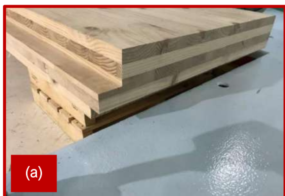
Figure 114: 210 mm thick five-layer Red Stag CLT panel with lap joint installed in the acoustic chamber at the testing laboratory.
