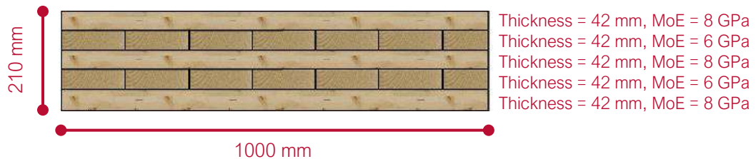
Figure 101: Red Stag CLT Panel Cross-Section
