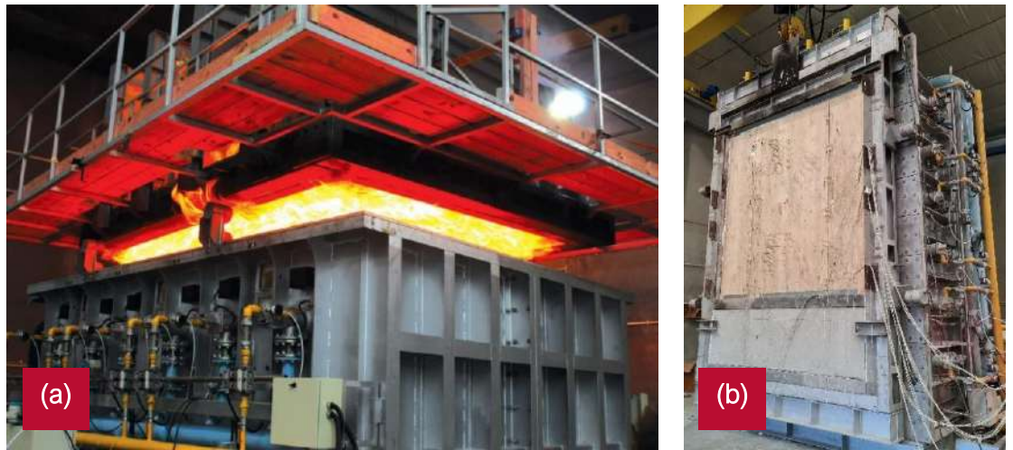
Figure 81: Large-scale fire testing on Red Stag EWP conducted by BRANZ; (a) Red Stag CLT floor test specimen after fire testing; (b) Red Stag CLT wall test specimen before fire testing.
