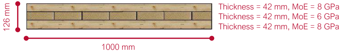
Figure 107: Red Stag CLT Panel Cross-Section
