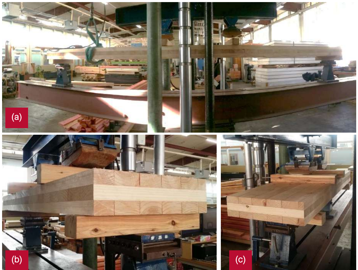
Figure 8: Large scale mechanical testing conducted by SCION; (a) Long span testing, (b) Median span testing, (c) Short span testing.
