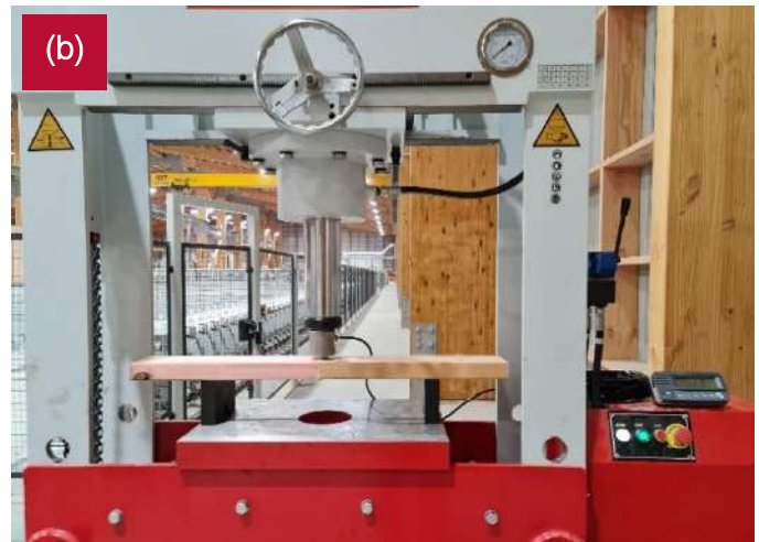
Figure 13: Finger joint test equipment and setup.
