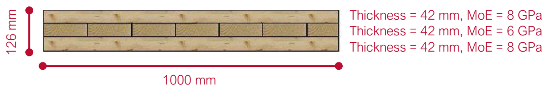
Figure 109: Red Stag CLT Panel Cross-Section
