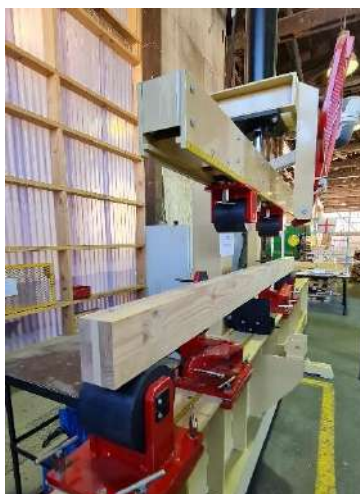
Figure 14: CLT beam bending testing machine and setup; (a) Isometric end elevation; (b) Front elevation.
