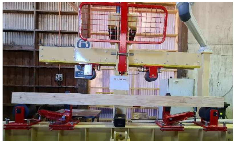
Figure 14: CLT beam bending testing machine and setup; (a) Isometric end elevation; (b) Front elevation.
