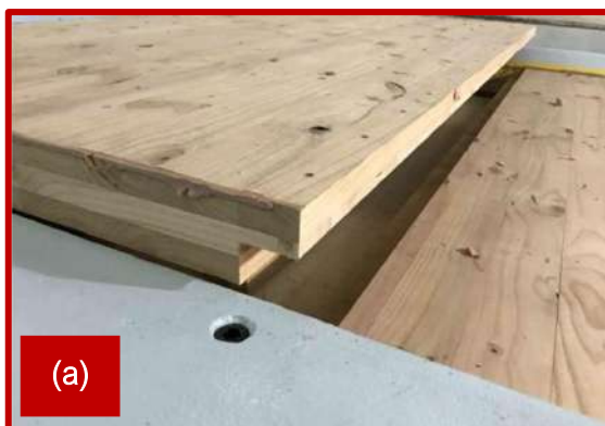
Figure 113: 126 mm thick three-layer Red Stag CLT panel with lap joint installed in the acoustic chamber at the testing laboratory.
