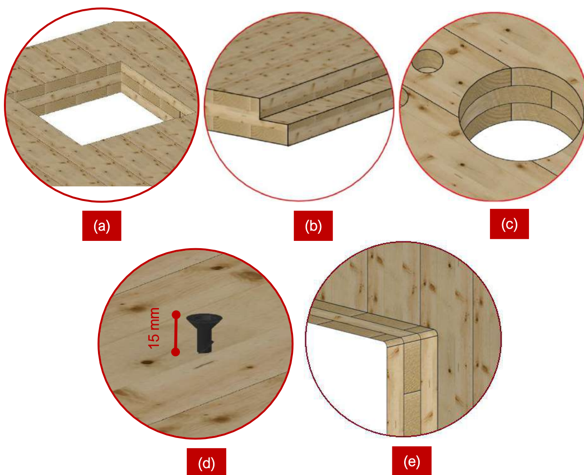
Figure 86: Example of very difficult complexity processing of Red Stag EWP elements; a) Up to three square cut outs (subject to minimum size for tooling); b) Lap/spline joint rebate without flipping or panel removal up to 120 mm wide; c) Up to six simple radii penetrations over and above of basic fixing locators; d) Predrilling/installation of lifting screws; e) Door or window corner on Red Stag CLT Wall Panel (either four radii openings or three-square openings).
