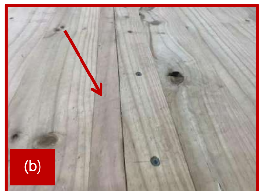
Figure 113: 126 mm thick three-layer Red Stag CLT panel with lap joint installed in the acoustic chamber at the testing laboratory.
