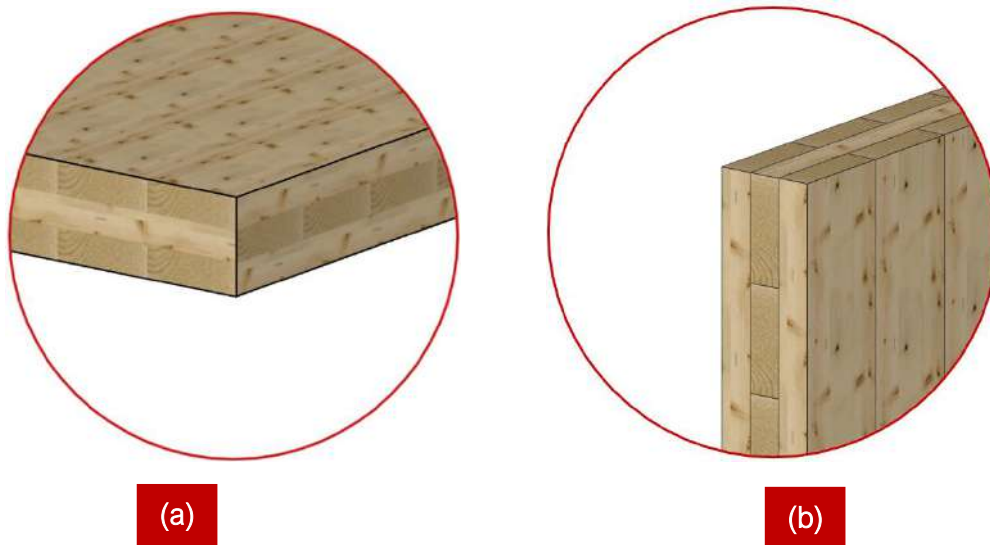
Figure 82: Example of basic complexity processing of Red Stag EWP elements; a) Corner of basic complexity Red Stag CLT floor panel; b) Corner of basic complexity Red Stag CLT wall panel.
