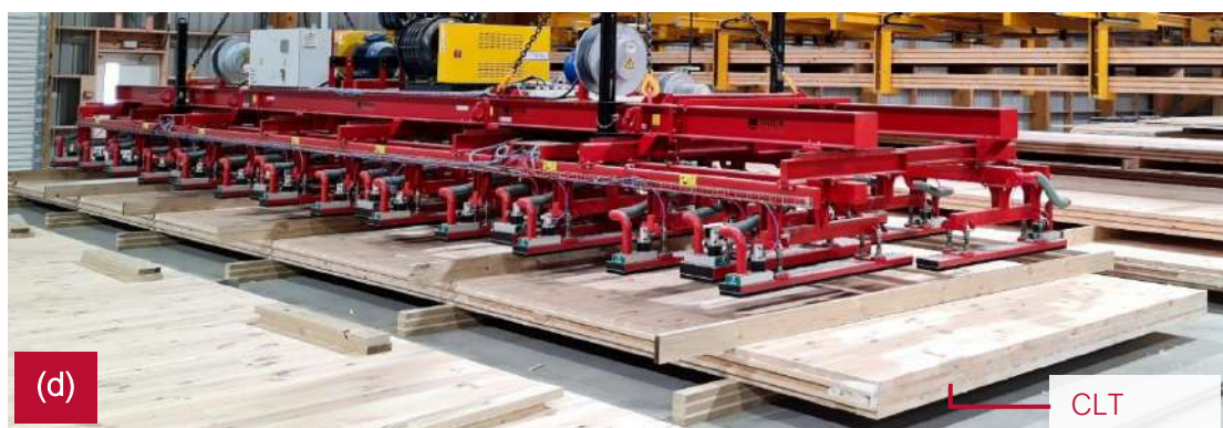
Figure 48: Red Stag's EWP manufacturing facility; a) panoramic view of the Red Stag remanufacturing line; (b) 16.5 meter lamella out of the Finger Joints (FJ) line; (c) EWP laminating equipment; (d) EWP material handling equipment.
