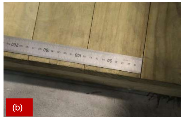
Figure 63: Red Stag CLT system and lamella dimensions.
