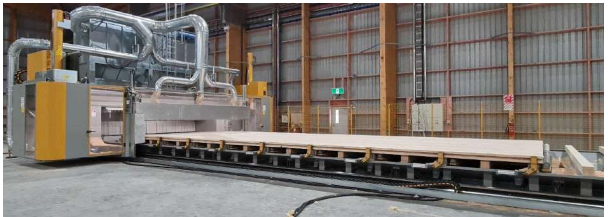
Figure 2: Precision large scale timber CNC processing equipment.
