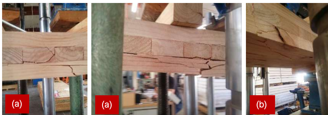
Figure 58: Failures in large scale CLT bending tests; (a) Rolling shear failure; (b) Tension failure.
