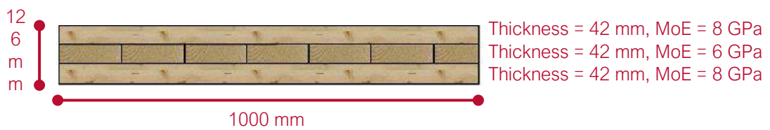
Figure 55: Red Stag CLT Panel Cross-Section.
