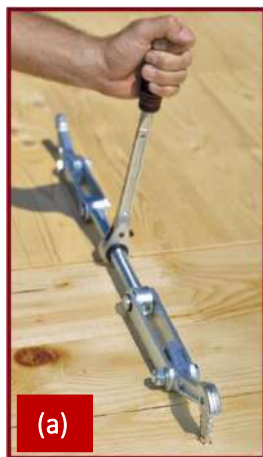
Figure 88: SKORPIO applications; a) SKORPIO utilised to pull CLT floor panels together; b) SKORPIO utilised to pull CLT wall panels together (pulling into a corner) [20] .
