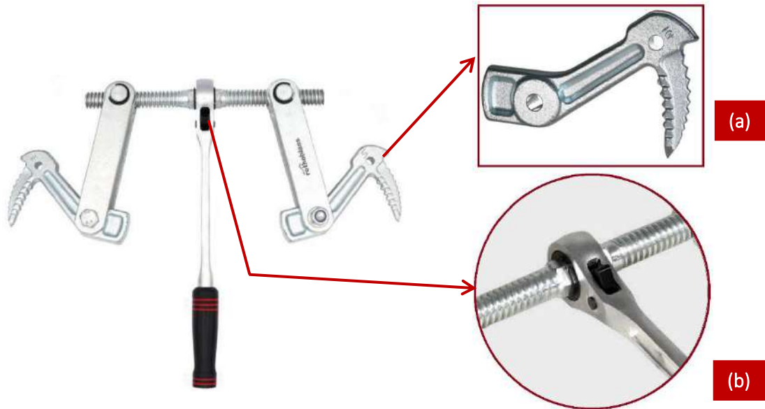
Figure 87: Components of a SKORPIO; a) Hammered in hook at each end; b) Reversible ratchet with sturdy fine thread to allow for fine adjustment [20] .
