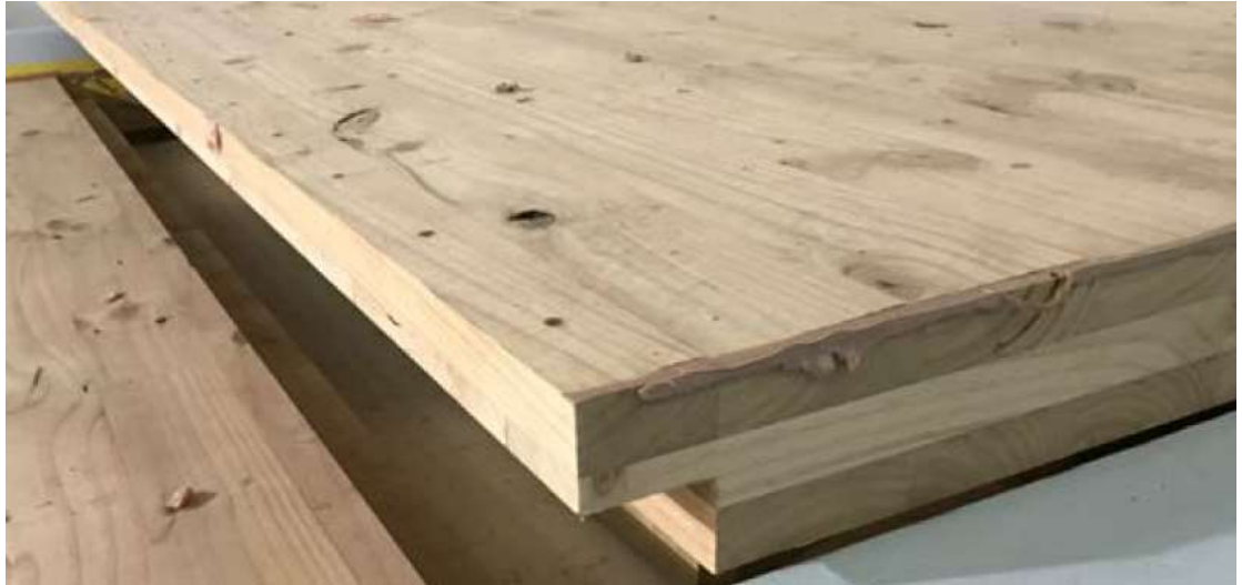
Figure 125: Three-layer Red Stag CLT panel with lap joint.
