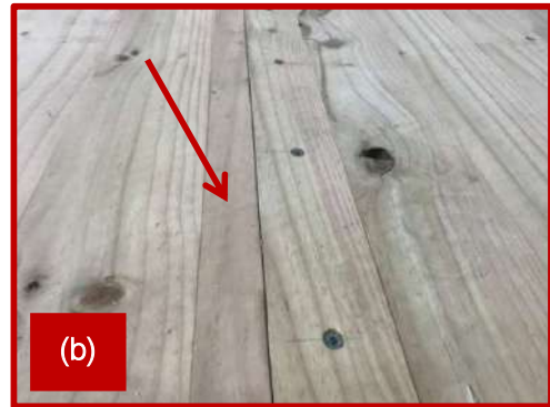
Figure 123: 126 mm thick three-layer Red Stag CLT panel with lap joint installed in the acoustic chamber at the testing laboratory.
