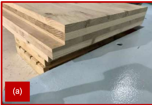
Figure 124: 210 mm thick five-layer Red Stag CLT panel with lap joint installed in the acoustic chamber at the testing laboratory.
