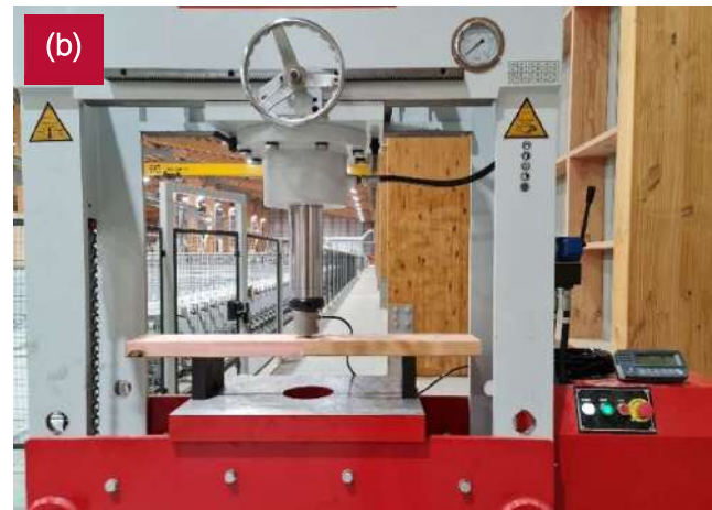
Figure 20: Finger joint test equipment and setup.
