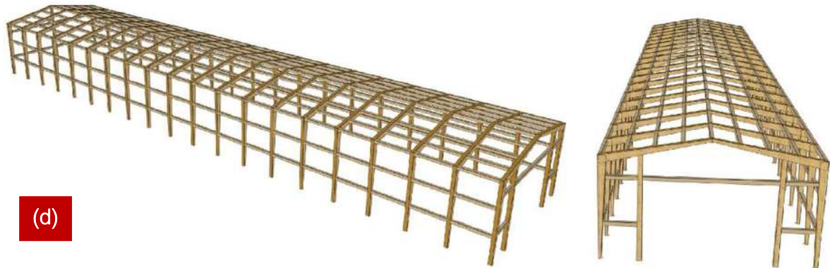
Figure 168: Fast and efficient CNC processing of Red Stag CLT portal frames; a) Optimisation process of CLT portal frame manufacturing; b) Red Stag CNC equipment; c) Parallel CLT portal frame at Red Stag stacker building; d) Truncated CLT Portal frame.
