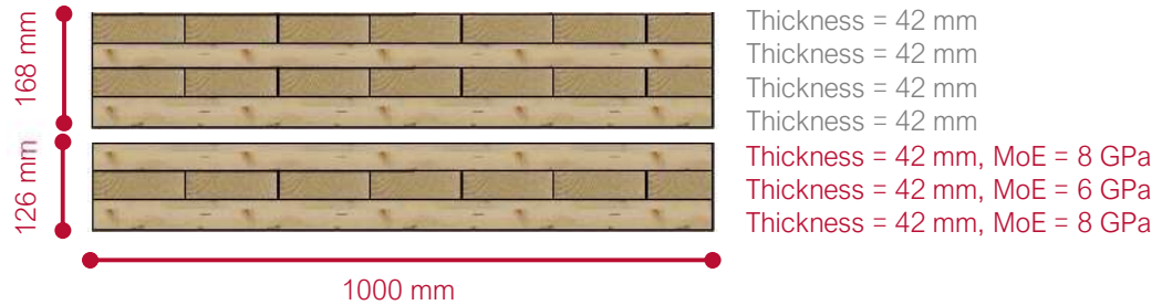
Figure 115: Red Stag CLT Panel Cross-Section
