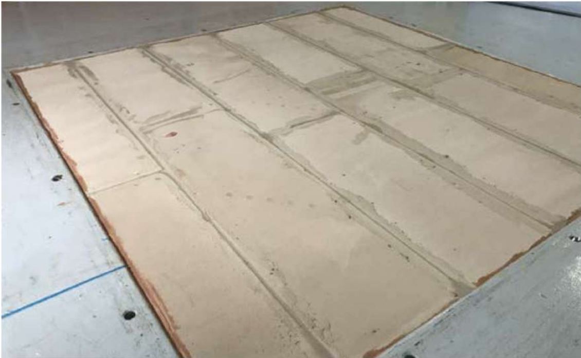
Figure 132: Sample installed in the chamber with tapping machine.
