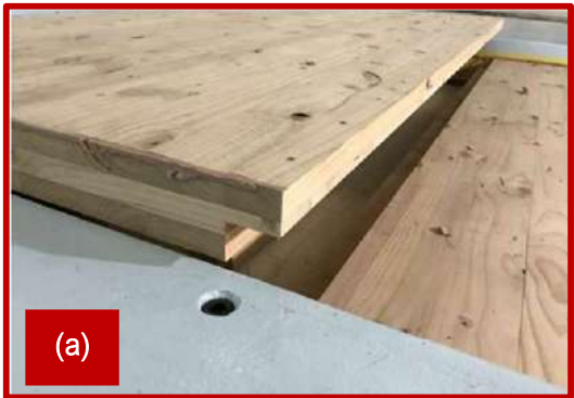
Figure 123: 126 mm thick three-layer Red Stag CLT panel with lap joint installed in the acoustic chamber at the testing laboratory.
