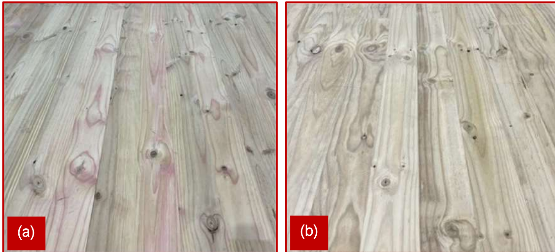
Figure 141: Example of surface on standard grade EWP; a) H1.2 Treatment; b) H3.2 Treatment.
