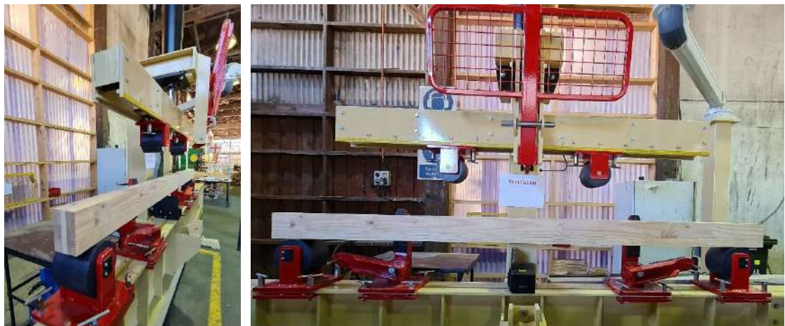
Figure 21: CLT beam bending testing machine and setup; (a) Isometric end elevation; (b) Front elevation.
