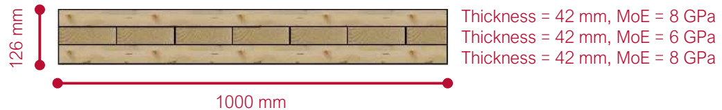
Figure 119: Red Stag CLT Panel Cross-Section
