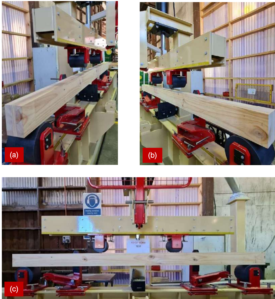
Figure 160: Large-scale mechanical testing of Red Stag CLT beams conducted by Red Stag; a & b) End Elevation; c) Elevation.
