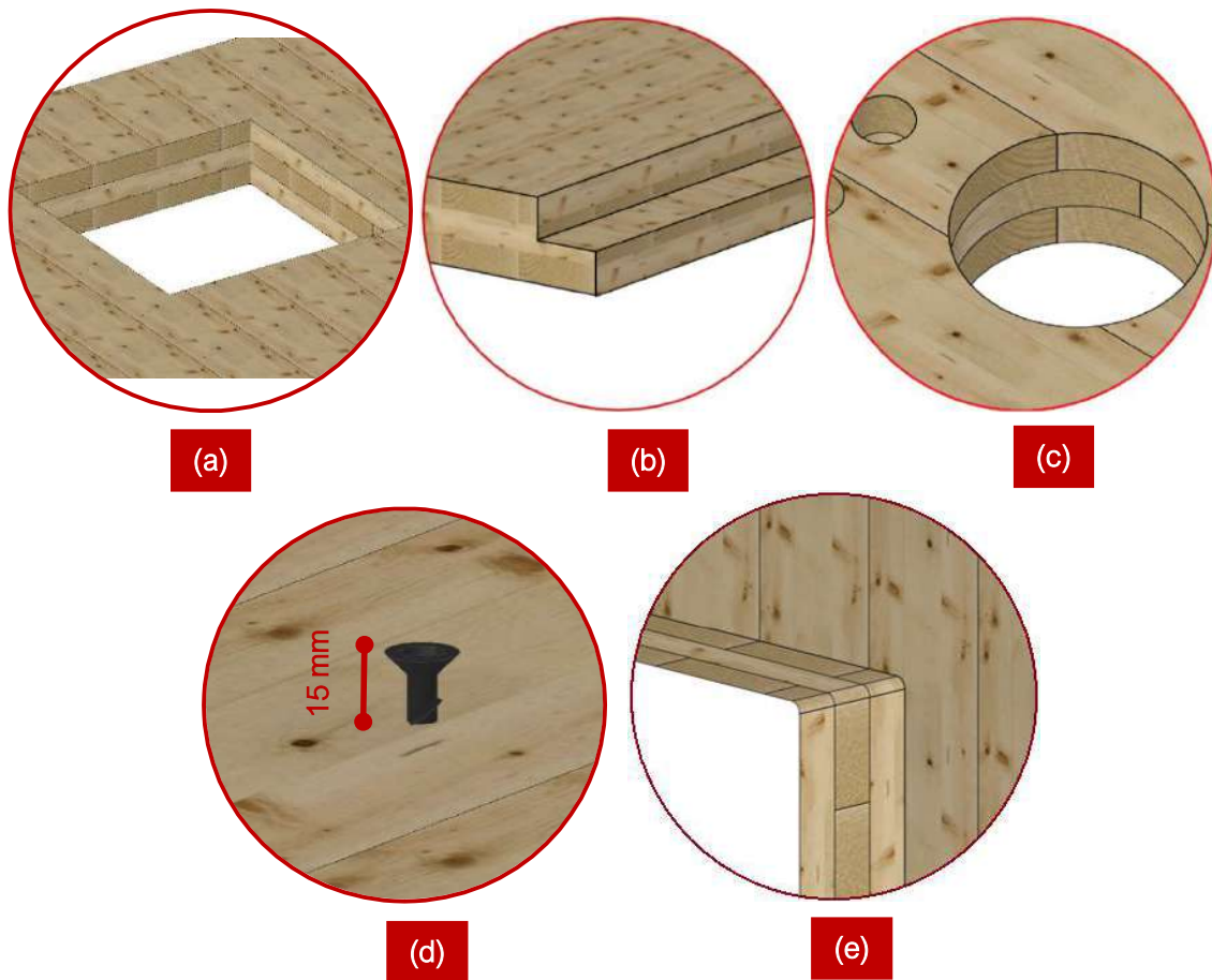
Figure 96: Example of very difficult complexity processing of Red Stag EWP elements; a) Up to three square cut outs (subject to minimum size for tooling); b) Lap/spline joint rebate without flipping or panel removal up to 120 mm wide; c) Up to six simple radii penetrations over and above of basic fixing locators; d) Predrilling/installation of lifting screws; e) Door or window corner on Red Stag CLT Wall Panel (either four radii openings or three-square openings).
