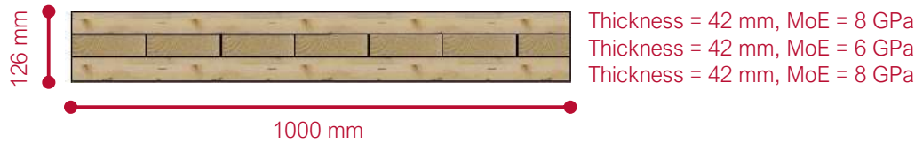
Figure 109: Red Stag CLT Panel Cross-Section
