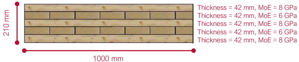
Figure 111: Red Stag CLT Panel Cross-Section
