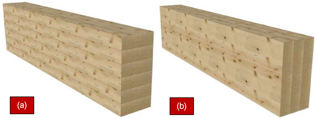
Figure 138: GLT 3D views; a) GLT horizontal brick layout; b) GLT vertical brick layout.
