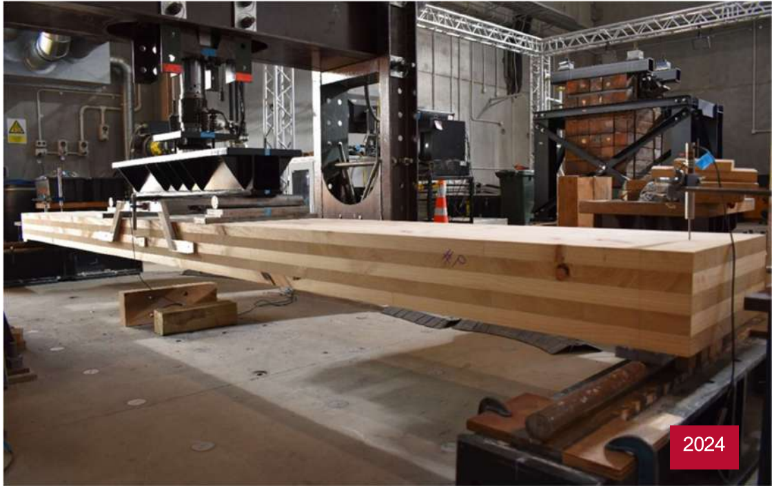
Figure 12: Large scale mechanical testing conducted by SCION; (a) Long span testing; (b) Median span testing; (c) Short span testing.
