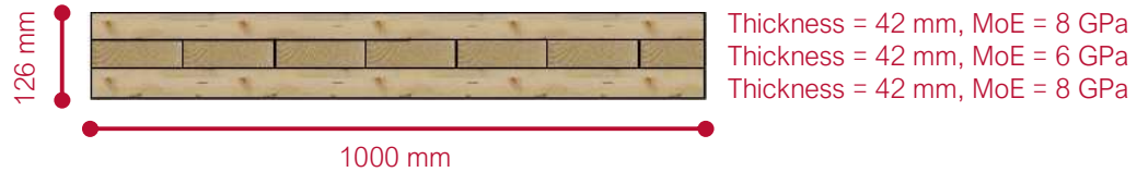
Figure 117: Red Stag CLT Panel Cross-Section
