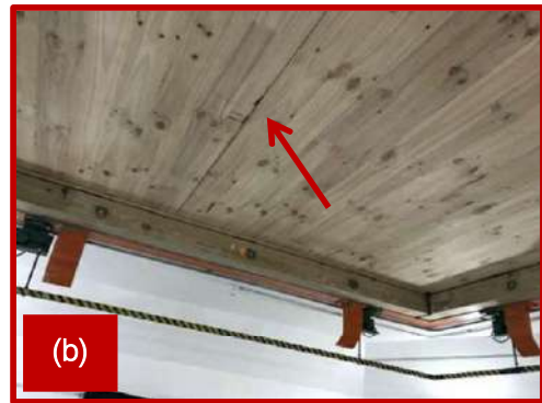
Figure 124: 210 mm thick five-layer Red Stag CLT panel with lap joint installed in the acoustic chamber at the testing laboratory.
