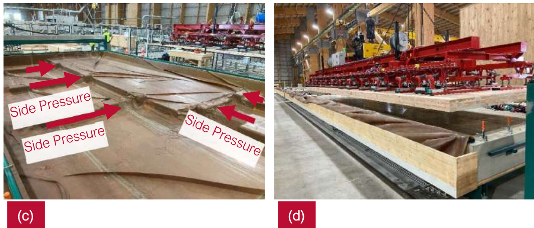
Figure 78: Red Stag Manufacturing line; (a) Layer arrangement with side pressure, (b) Adhesive distribution, (c) Hydraulic side pressure and Vacuum Membrane, (d) Final Red Stag CLT Product.
