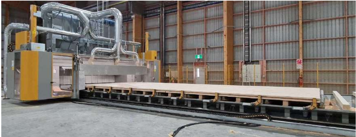
Figure 80: CNC equipment with precise cutting capability.
