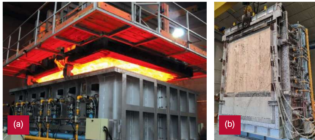
Figure 17: Large-scale fire test specimen set-up for the fire testing on Red Stag CLT; (a) Red Stag CLT floor test specimen after fire testing; (b) Red Stag CLT wall test specimen before fire testing.
