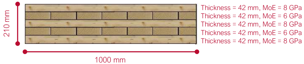
Figure 113: Red Stag CLT Panel Cross-Section
