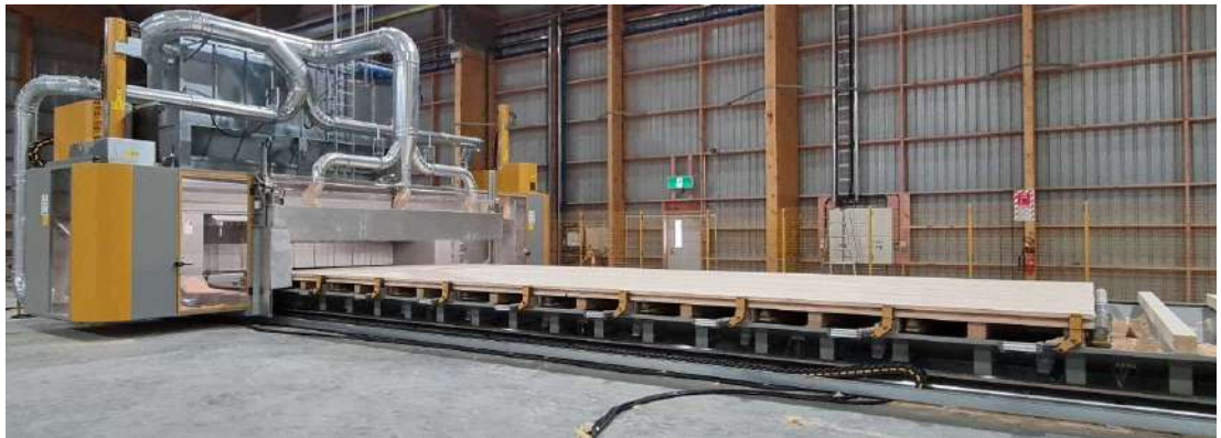
Figure 2: Precision large scale timber CNC processing equipment.
