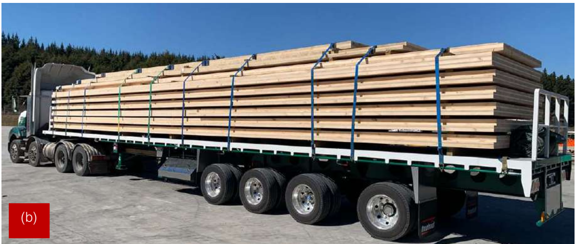
Figure 5: Example of truck loading configuration; (a) Detail of truck loading, (b) Actual truck loading from Red Stag projects.
