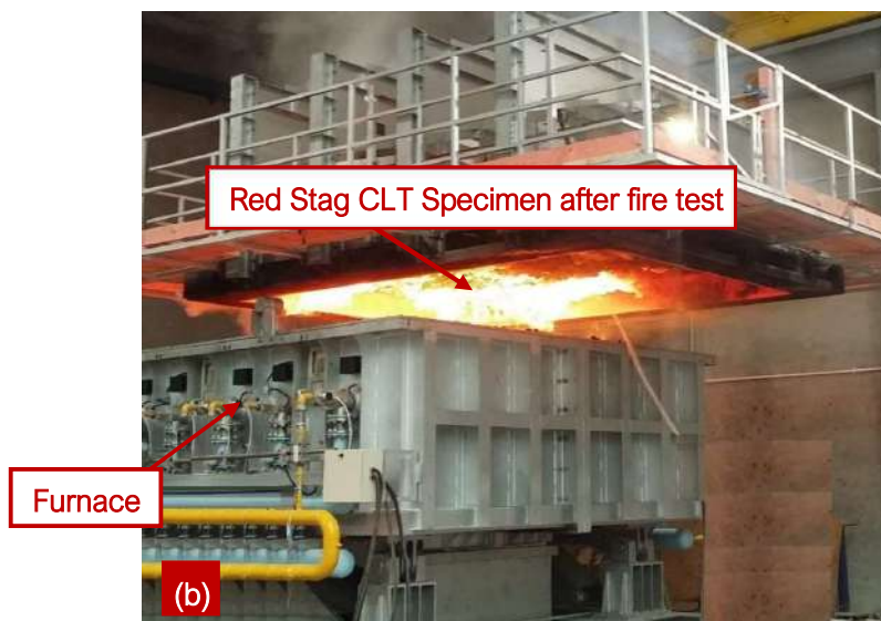
Figure 64: 103.5 mm thick Red Stag CLT Specimen; (a) Test specimen before the fire test; (b) Large scale fire test setup and specimen after fire test.
