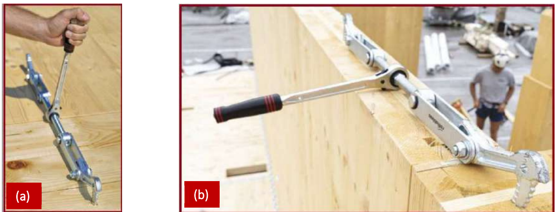
Figure 88: SKORPIO applications; a) SKORPIO utilised to pull CLT floor panels together; b) SKORPIO utilised to pull CLT wall panels together (pulling into a corner) [20] .
