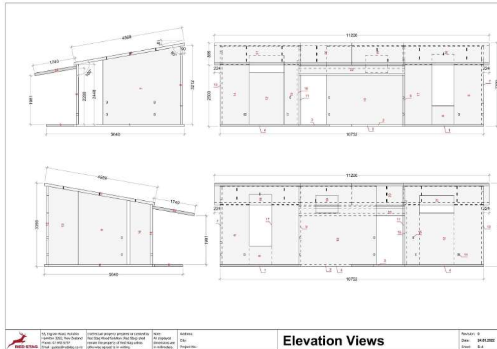
Figure 8: Example of Red Stag shop drawing elevations.
