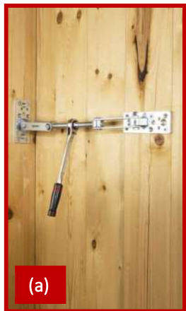
Figure 90: GEKO applications; a) GEKO utilised to pull CLT wall panels together (pulling into a corner); b) GEKO utilised to pull CLT floor panels together [21] .
