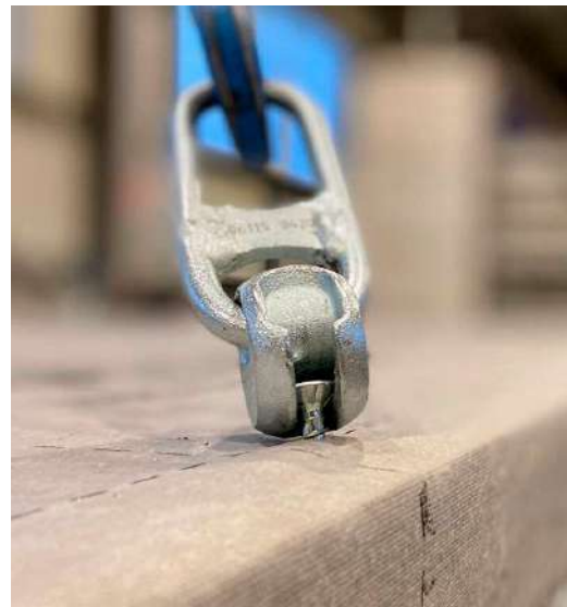
Figure 16: Screwed anchor lifting components.
