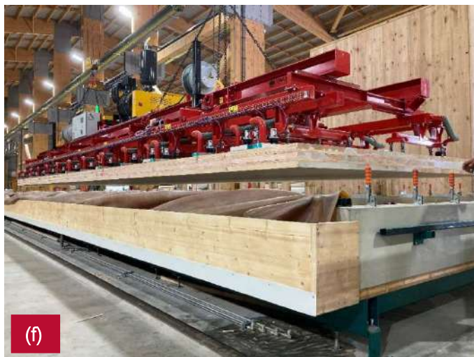
Figure 54: (a) Red Stag CLT gluing process; (b) Gluing laser alignment system; (c) Short lamella layup; (d) Clock/timer to log open and close times; (e) Panel under vacuum; (f) Cured laminated EWP billet being removed from press.
