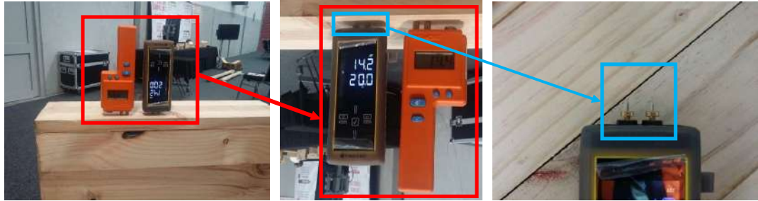
Figure 52: Moisture content measurement of the EWP lamella with suitable timber moisture meters (resistive meters illustrated, but capacitance meters are also acceptable).
