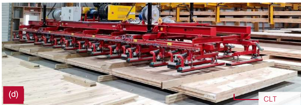
Figure 48: Red Stag's Rotorua EWP manufacturing facility; a) panoramic view of the remanufacturing line; (b) 16.5 meter lamella out of the Finger Joints (FJ) line; (c) EWP laminating equipment; (d) EWP material handling equipment.
